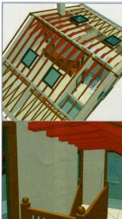
Figure 2: A more modern example of an application of 3D CAD of a conversion of a family house to transform loft space into more accommodation.
